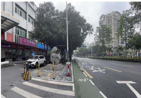
■ Figure 6-21 Narrow Bike Lane and Missing Physical Separators on Some Road Sections
