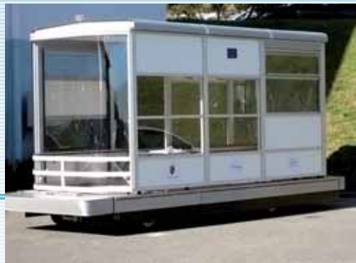
Cyberbus developed by Robosoft for use at the new Rome Exhibition Centre
