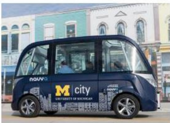
Navya's self-driving shuttle bus can travel back and forth along a two-mile route at the University of Michigan
