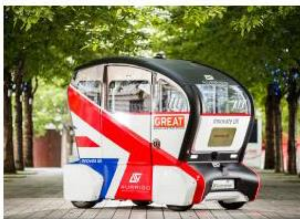
The UK Autodrive pod developed by RDM. 40 vehicles will operate fully autonomously in a public trial to be held in Milton Keynes city centre during summer 2018
