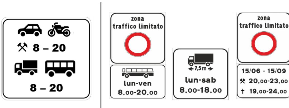
Figure 14: Supplementary panels for time validity, examples from France (optimised - left), and Italy (existing vs. optimised - right).
