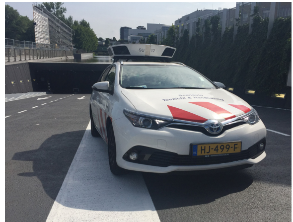
Figure 23. Scan car in Rotterdam (Park4SUMP, 2019)
