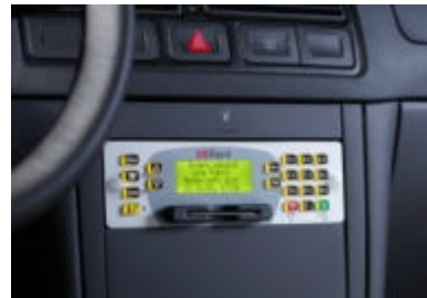
Fig. 8 Onboard Computer Standalone System "BCSA"
