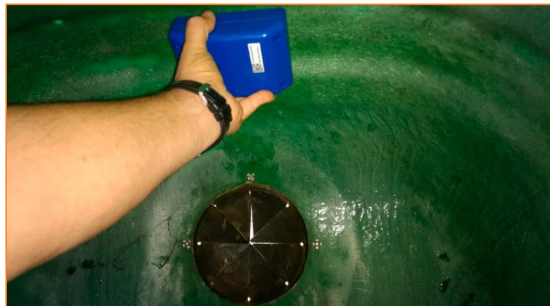
Figure 7 Sensor inside a glass container. Best practice from the Municipality of Calatayud. Taken from the European project Synchronicity 15
