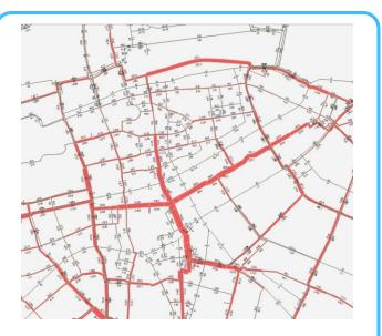
Figure 2: An example of the output from the bicycle model that shows today's cycle flows based on today's cycling network. The bandwidth is proportional to the traffic flow (graphic provided
