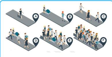
Figure 3: Illustration of pedestrian Level of Service
