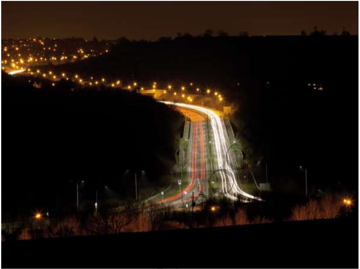
Figure 3-12: Luminaires with ULOR=0 in the bottom part of the picture and emitting light upwards in the top part. (Source: Philips, Hicksgate case study)
