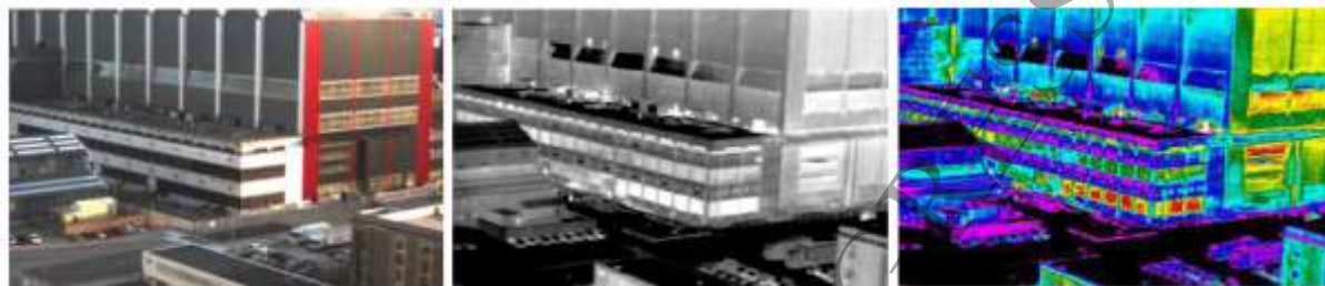
Figure 3-43: example of land-based thermographic imaging (source TCC sas)
