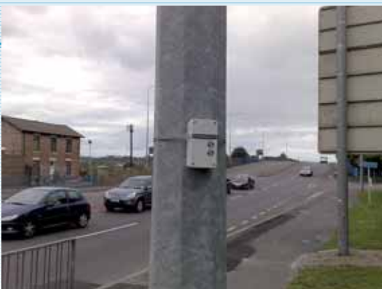
Lamp post-mounted wireless sensor for monitoring NO x , CO, noise, temperature and humidity Photo: UNEW
