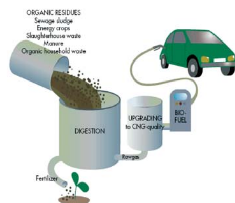
Lille: from organic residue to tank, the biogas cycle
