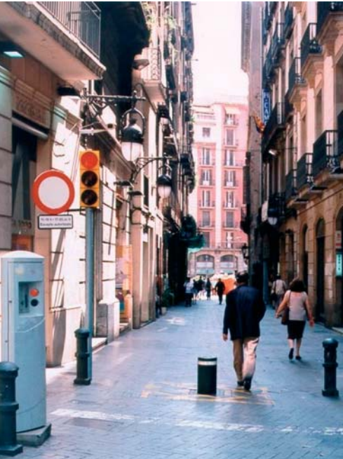
Barcelona: access restriction with retractable bollards
