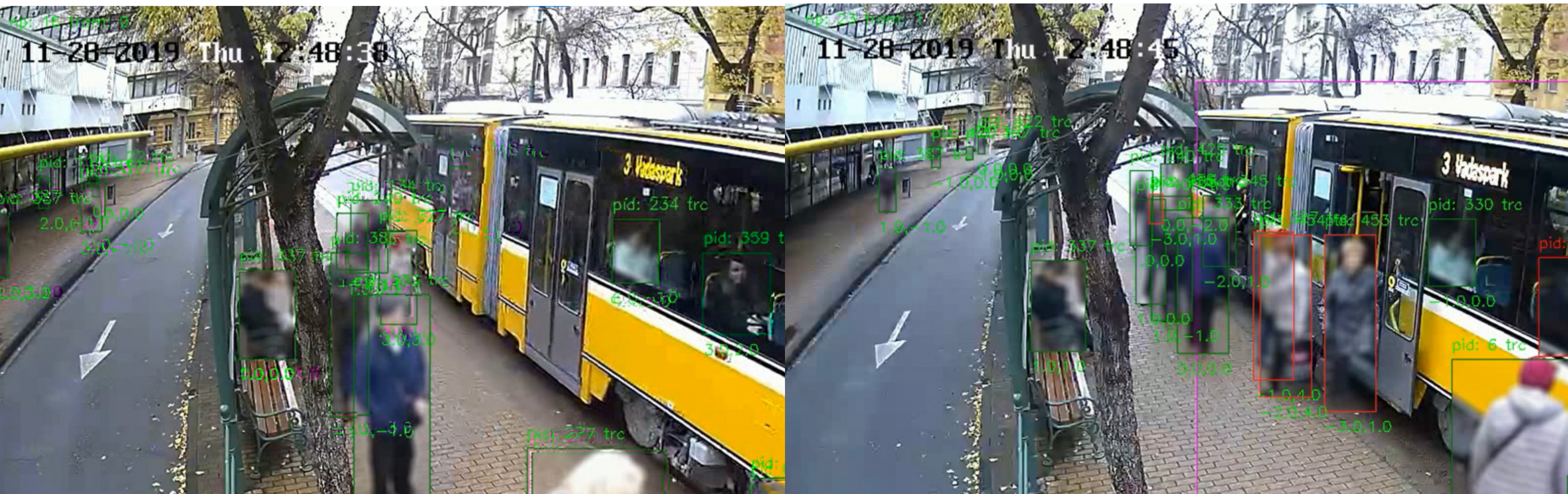
Stills from live video feed showing real-time passenger counting (SZKT, 2020)
