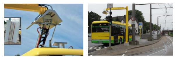
Figure 9 - Pantograph on top of the SOLARIS Bus Roof and Charging Infrastructure at the Station Neumarkt (source: STOAG)
