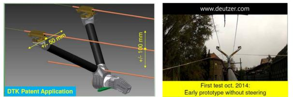
Figure 19 – Automatic wiring system from Deutzer
