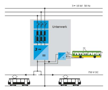
Figure 8 – Schematic Sketch of the Bus Charging from the Tram Sub-station at the Station Neumarkt (source: Müller-Hellmann)
