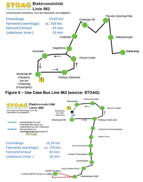
Figure 7 – Use Case Bus Line 966 (source: STOAG)
