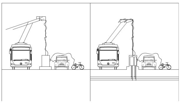
Figure C 7 - Diagram of the planned multi-purpose e-vehicle charger
