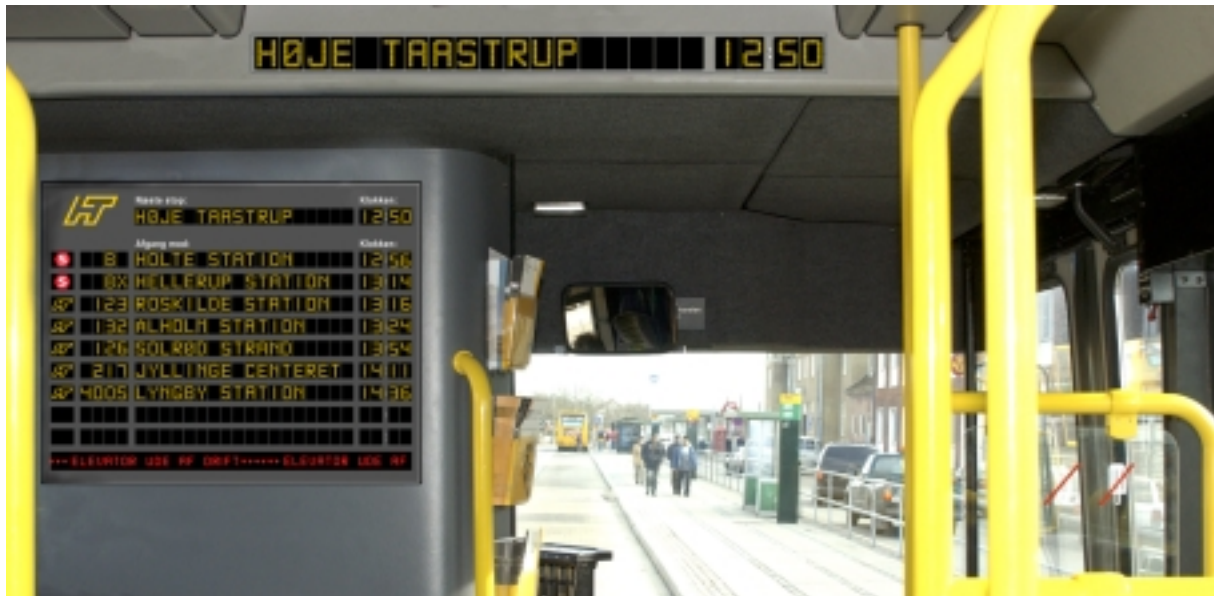
Figure 1.3: Improved passenger information systems in public transport vehicles
