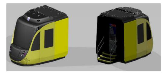
Figure 3: Full cabin simulator 2. generation, VBK Stadtbahn, view presentation via monitors, seat shaker
