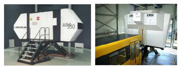
Figure 1 and 2: Full cabin simulators (1. generation): BVG-Tram (left), SSB-AG Stadtbahn (right), view presentation via projection, 6 DOF electromechanical moving system
