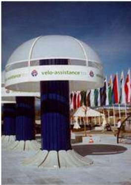
Bike Tree: 12 bicycles are hung on their front wheel. 30% of space is saved.
